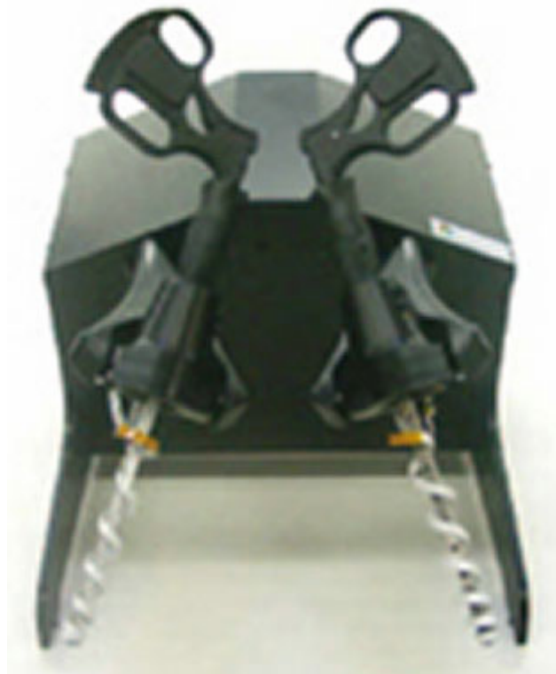
Figure 2.12. The Laparoscopic Surgical Workstation, a haptic device for the simulation of laproscopic surgery (reprinted without permission from www.immersion.com ).
