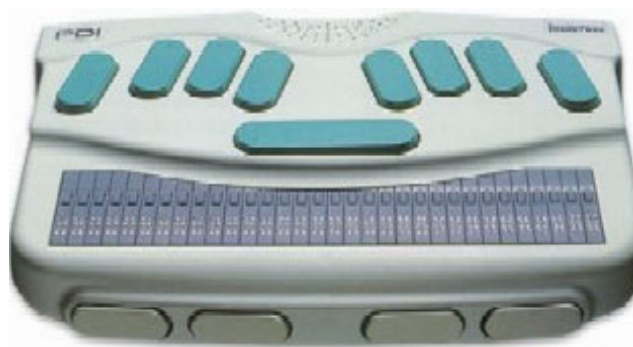
Figure 2.3. The Braillenote, a tactile display for visually impaired users (reprinted without permission from www.brailnote.com ).
