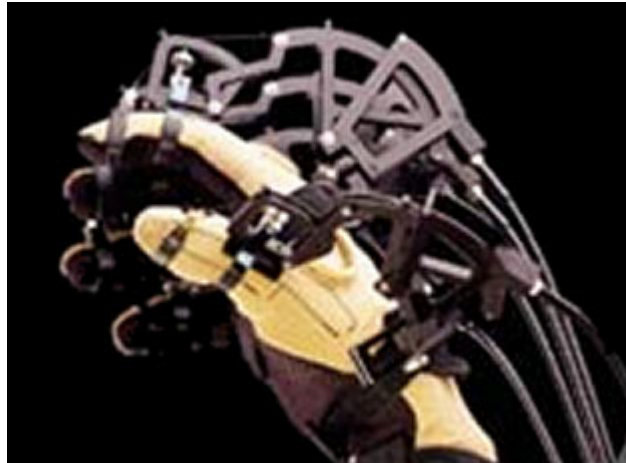
Figure 2.11. The Cybergrasp glove based force feedback device (reprinted without permission from www.immersion.com ).
