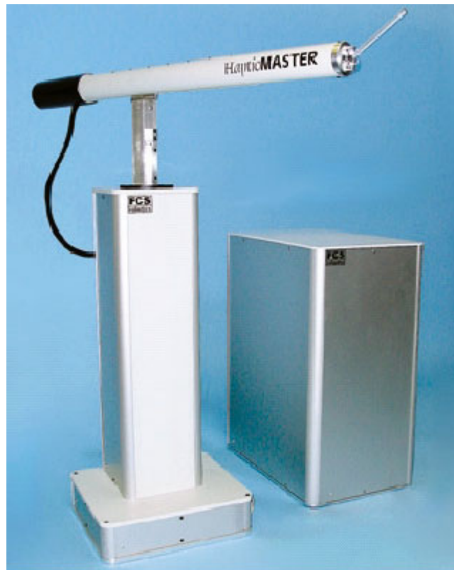
Figure 2.7. A typical ground based haptic device, the HapticMaster (reprinted without permission from www.fcs-cs.com/robotics/ ).
