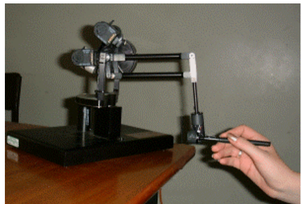
Figure 1: The Phantom 3D force feedback device from SensAble Technologies. The stylus shown has a button that can be used for performing the mouse clicks in the experiments reported.
