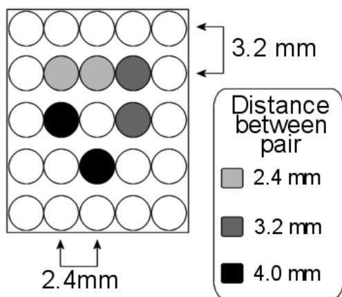
Figure 4. Diagram of pneumatic array showing sample set of stimuli used in second two point threshold study.
