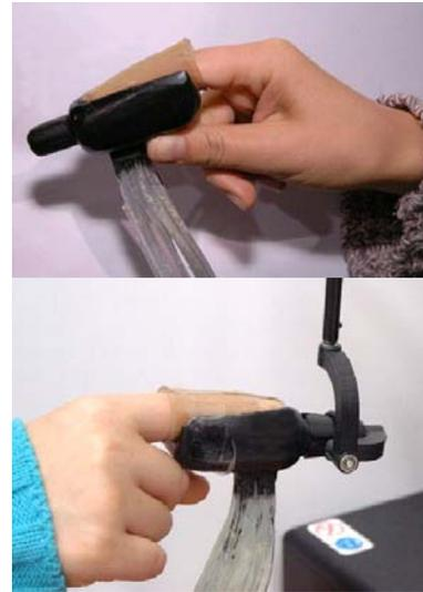
Figure 10. Pneumatic array housing for easy attachment to PHANToM force feedback device.
