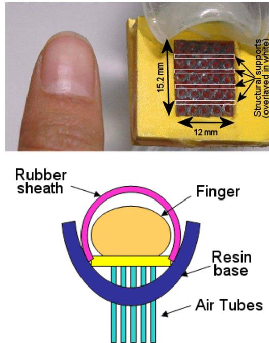
Figure 1. Photograph and schematic of initial prototype of pneumatic array.
