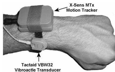
**Fig 4.** X-Sens MTx and Tactaid VWB32 used to produce WristMenu prototype
