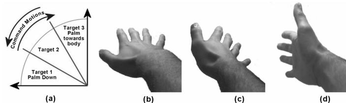
**Fig 1.** General control scheme for motions (a) and the three specific hand/forearm poses used in the system: selecting target 1 (b), target 2 (c) and target 3 (d).
