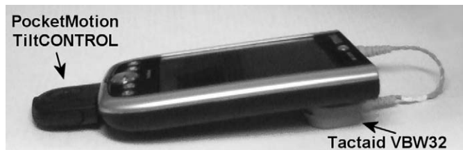
Fig. 4. Final experimental device, showing motion sensor and vibrotactile transducer.
