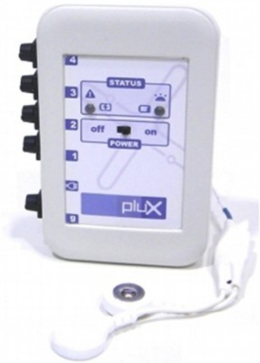
Figure 1. bioPLUX biosignal acquisition device. The bioPLUX system for clinical biofeedback applications features Bluetooth connectivity and four input channels, allowing real-time wireless monitoring of up to four muscles via EMG and display of interactive feedback relating to this activity on a base station, where both patients and practitioners can visualize the work being done and main outcomes.
